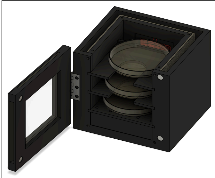
Figure C.5: Double Wall Insulation Design
